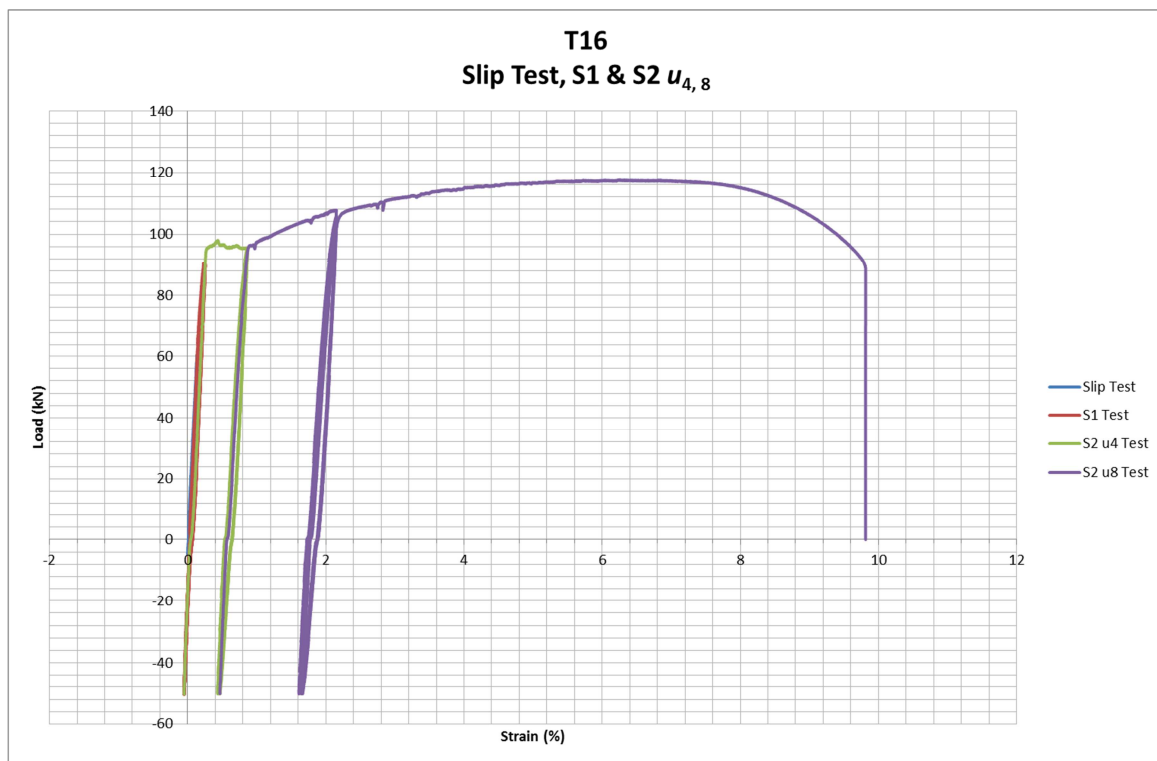
G1. T16 Alternating tension and compression test of large stresses (S1) and large strains (S2) in the mechanical splice - Load vs Strain Graph
