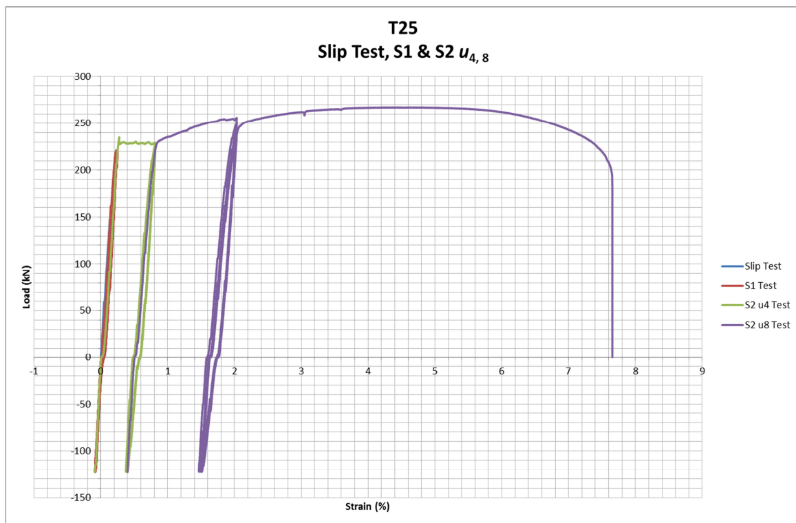
G2. T25 Alternating tension and compression test of large stresses (S1) and large strains (S2) in the mechanical splice - Load vs Strain Graph
