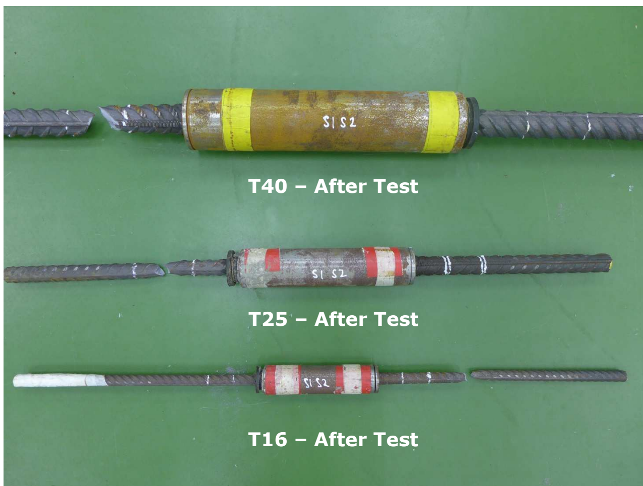
P2. T16, T25 & T40 Alternating tension and compression test of large stresses (S1) and large strains (S2) in the mechanical splice (After Test)
